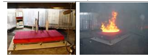
[DS1 at the beginning and at 4 min 30 s] - Max HRR of 429.49 kW - Max SPR of 42.03 m 2 /s
