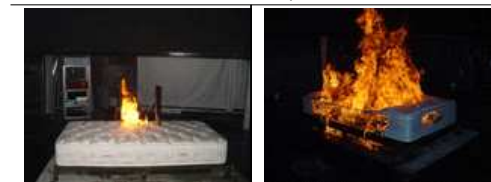
[SS1 at the beginning and at 4 min 30 s] - Flashover occur - Max SPR of 6.66 m 2 /s
