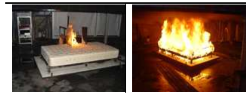
[AS1 at the beginning and at 4 min 30 s] - Flashover occur - Max SPR of 41.56 m 2 /s
