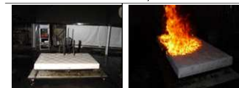
[RS1 at the beginning and at 4 min 30 s] - Max HRR of 447.93 kW - Max SPR of 9.81 m 2 /s
