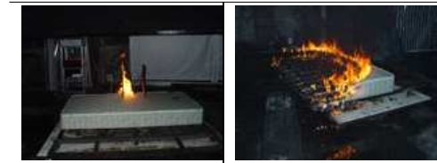
[PS1 at the beginning and at 4 min 30 s] - Max HRR of 146.16 kW - Max SPR of 3.42 m 2 /s
